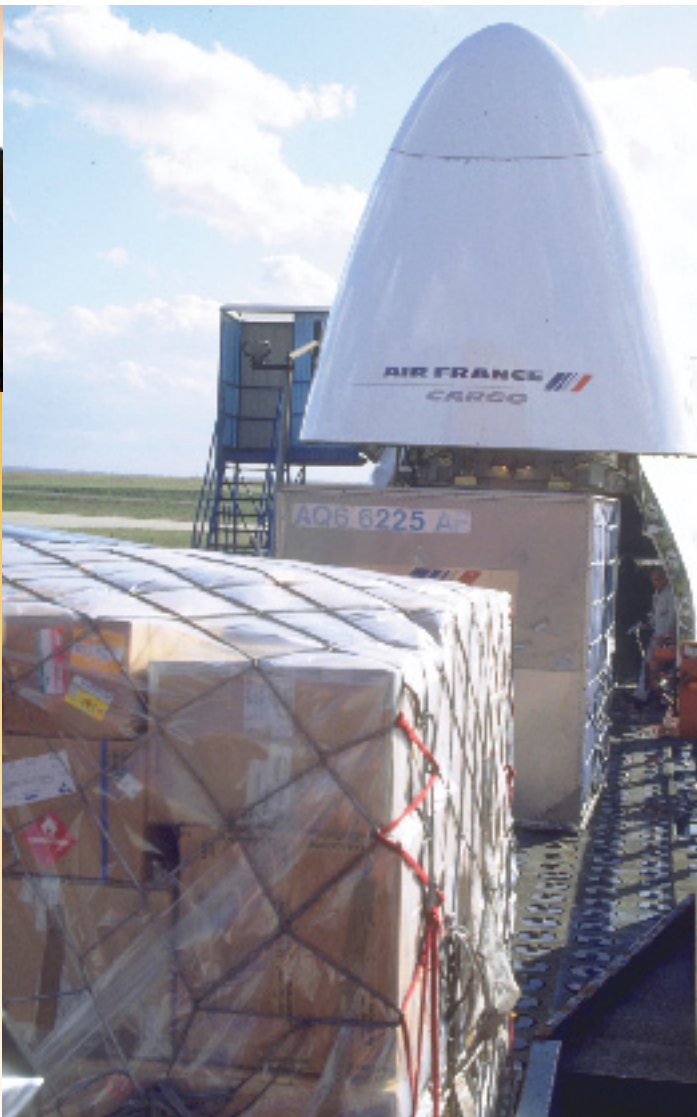
Loading of pallets by the nose door of the "Super Pelican"
