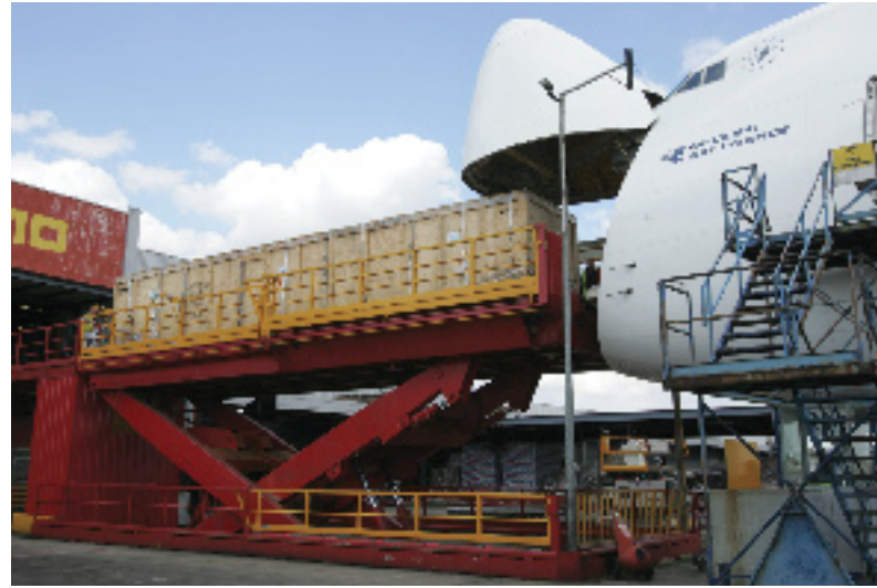
Loading of an outsize shipment through the nose of the B747 freighter at Paris-CDG Airport
